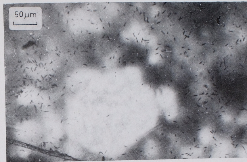
Phot. 1. Uranium distribution in basalt from Księginiki (sample 224). Fission fragment tracks of ^{235}\text{U} nuclei recorded in Estrofol foil. Uranium content in microcrystalline matrix is higher than in pyroxene phenocryst
